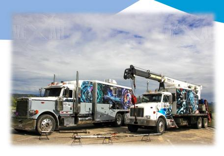
Model LV2-100 series is a tandem axle heavy duty van unit for open hole or case hole logging and perforating service work applications. This unit is designed to operate in arctic, desert and tropical oilfield environments and can be modified to perform other wireline service work applications.
